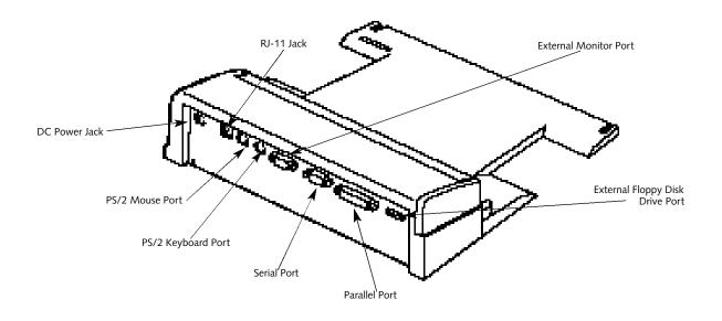
Figure 4-20 Port Replicator Rear View
